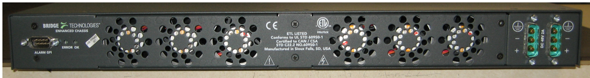
Figure 4.2: ECDC rear: two –48V DC connectors located on the the right
